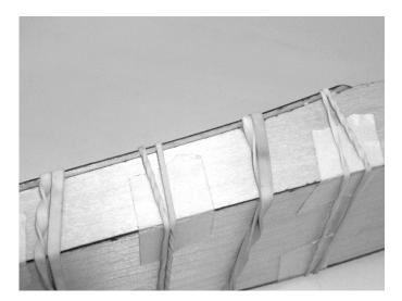
6. Glue (2) front tops to sides. Again, there will be about 1/16" overhang. Allow glue to partially dry. If wanted, put glue inside the hull and hang/rest it upside down to allow the glue to run up the inside corners. Allow glue to dry.
