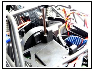
10. Mount Servo to servo mounts, reusing the(4) M3 screws that came with the Twin Hammers.
