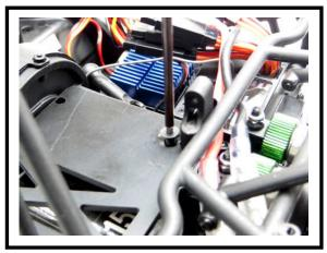
9. Install drilled-through servo mount through Shift Servo Plate and into transmission.
