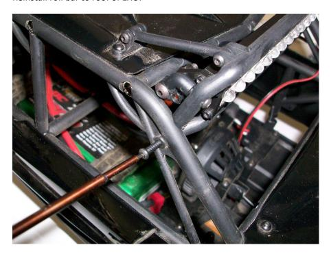
Connect Trail Torch LED light bar to any available port on your receiver or to a (3) or (4) AA or AAA battery holder. The light bar is designed to run on 4.5 to 6.0 volts.
