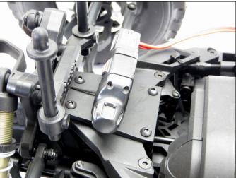
5. Using (4) of the M2 x 5mm Socket Head Screws, install roller fairlead (removed from 3Racing winch in Step 1) to SPACER.
