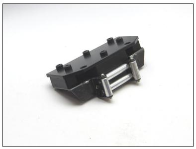
7. Attached roller fairlead assembly to Yeti front bumper using (2) M3 x 10mm and (2) M3 Lock Nuts:
