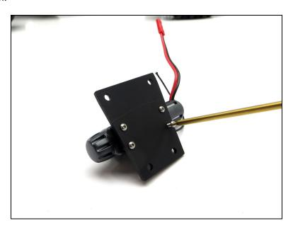
3. Remove the (4) flat head screws from the Yeti as shown:
